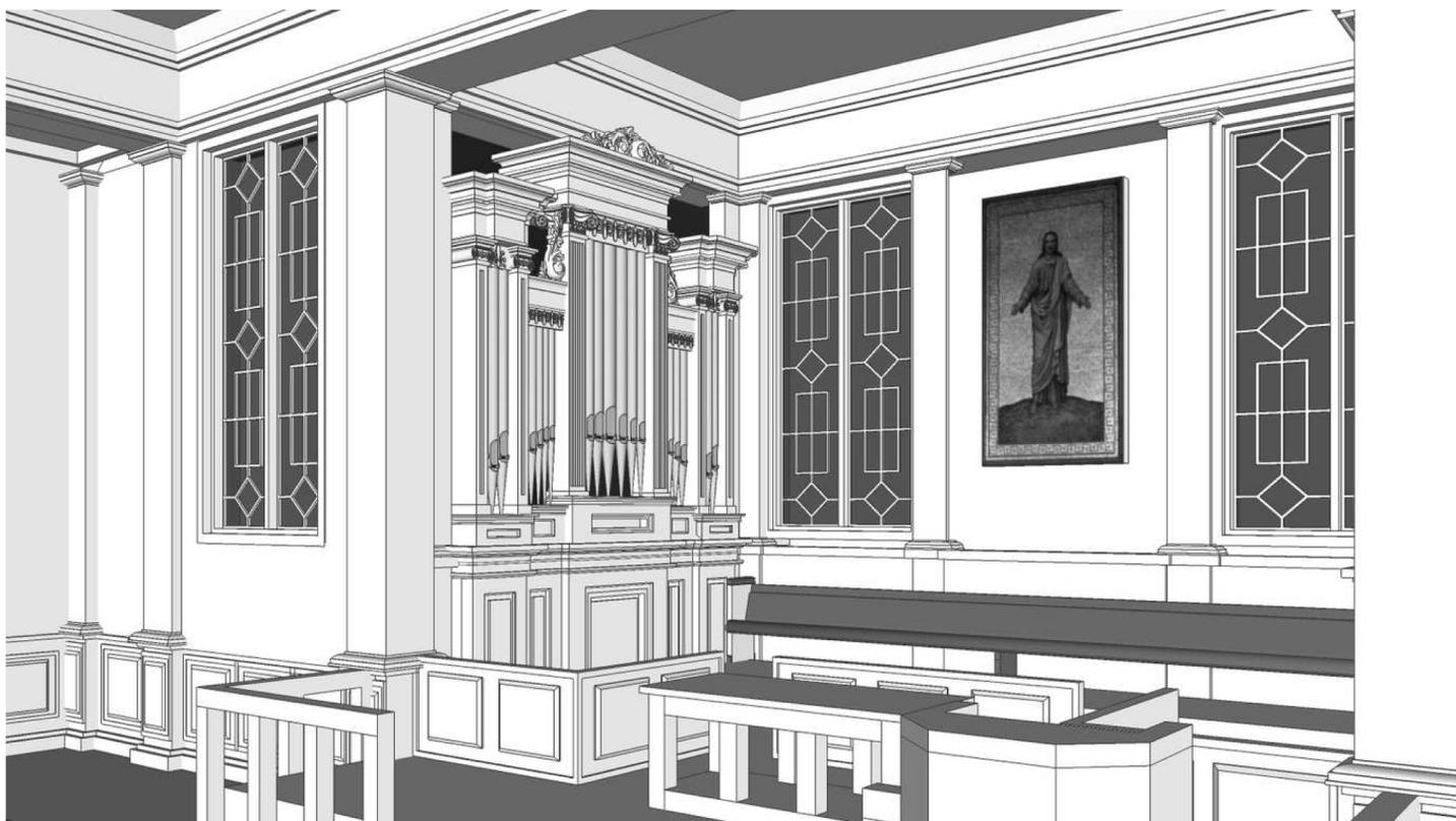
This 3-manual, 54 rank, electro-pneumatic organ has served faithfully since 1963. The entire organ has been moved to our shop for a major renovation including restoring the windchests; building a new state of the art console; adding manual and pedal ranks; revoicing existing ranks for a warmer sound; and creating two new Greek Revival style organ cases to harmonize with the church's gracious architecture.
