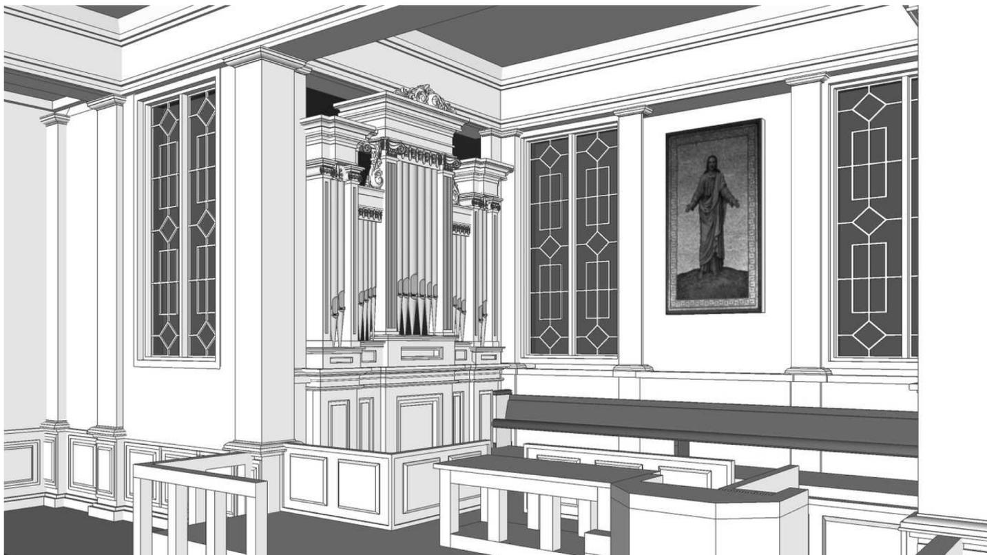
This 3-manual, 54 rank, electro-pneumatic organ has served faithfully since 1963. The entire organ has been moved to our shop for a major renovation including restoring the windchests; building a new state of the art console; adding manual and pedal ranks; revoicing existing ranks for a warmer sound; and creating two new Greek Revival style organ cases to harmonize with the church's gracious architecture.
